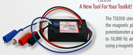
The TSE050 simulates a running engine when connected to the magnetic pickup input on a speed control. An on-board potentiometer allows the signal to be adjusted between 750 to 10,000 Hz and is compatible with all GAC speed controls using a magnetic pickup.
