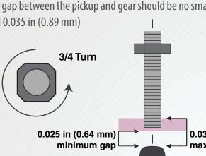
4. Wire leads should be twisted for their entire length from the magnetic speed sensor to the control unit. Shielding is required if external interference is present or the leads are longer than 10 ft (3 m).
